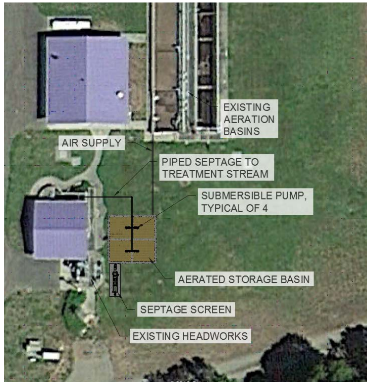
Figure 6.4 – Septage Receiving Preliminary Layout
