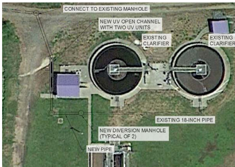
Figure 6.7a –Open Channel UV Disinfection
